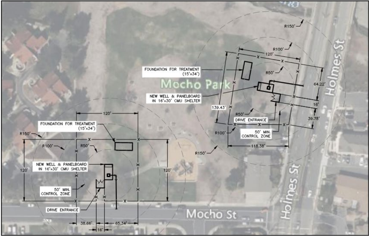
DETAIL 1 PURCHASE OPTION 1 & 2 PROPOSED SITE PLAN SCALE: 1" = 60'
